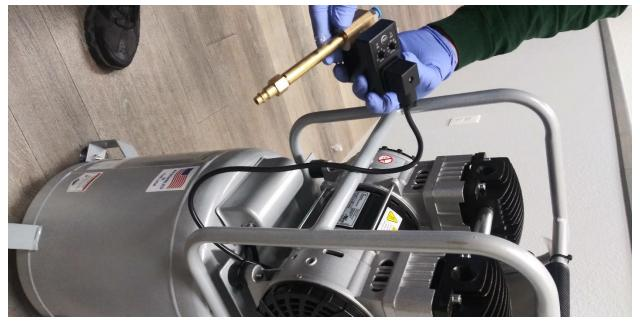
2. Ley unit down, stretch auto drain cord to the end of the tank.
