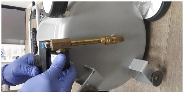
3. Tilt auto drain to the insert in to the quick connect, unit is ready to use. Drain unit from above to disconect auto drain if needed.
